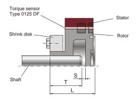
Total length of torque sensor: L - T + S (safety)
